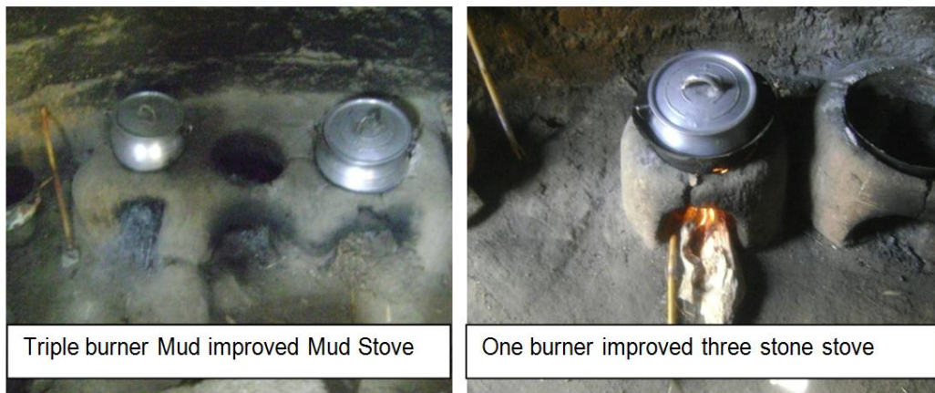
Fig. 3. Two versions of improved three stone fire stove; triple burners
