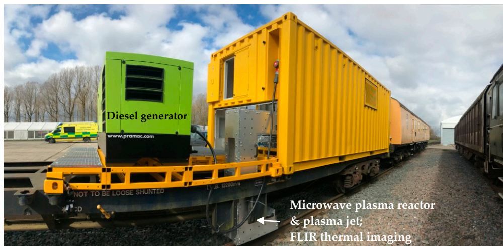
Figure 2. Photo of the mobile unit. Microwave generator, gas distribution and control systems mounted inside the yellow container. FLIR camera for thermal imaging mounted outside, targeting the contact between the plasma jet and the rail track. Videos of the laboratory and mobile on-track real condition testings have been uploaded in the supplementary files.
