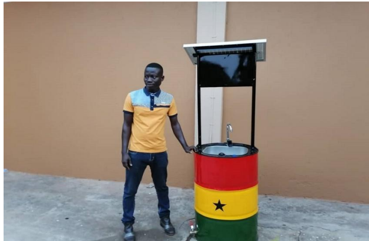
Fig. 1. A Solar-powered hand washing sink
