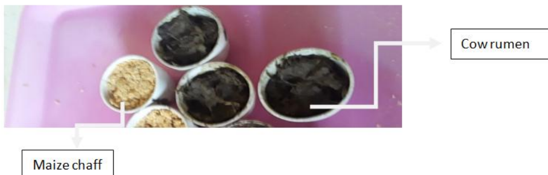
Fig. 1. Nature of the samples after 105°C Total Solid (TS) from the furnace
