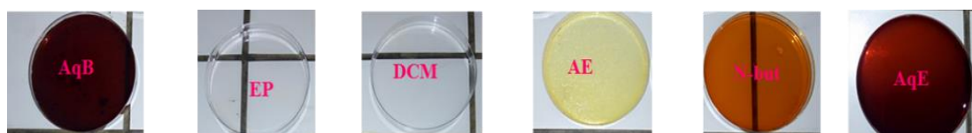
Fig. 6. The different extracts of dyes resulting from liquid-liquid separation; Aqueous crude (AqB), Petroleum ether (EP), Dichloromethane (DCM), Ethyl acetate (AE), N-butanol (N-but) and spent aqueous extract (AqE)
