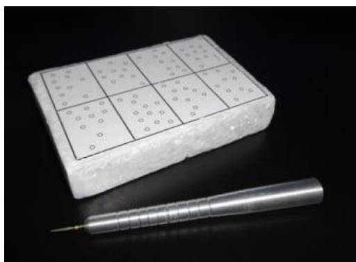
Fig. 1. Front and side view of the test cube and straight handpiece simulator with a #3195 diamond bur
